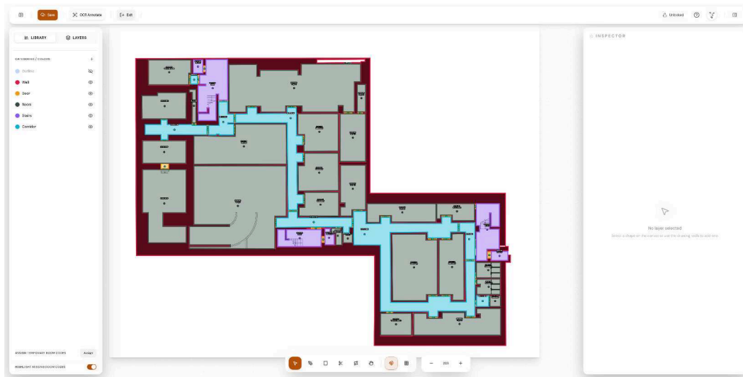
Figure 5.7 The main editor interface. Left panel: category legend with visibility toggles. Center: SVG canvas with the floor plan image and polygon overlay. Right panel: properties for the selected element.
