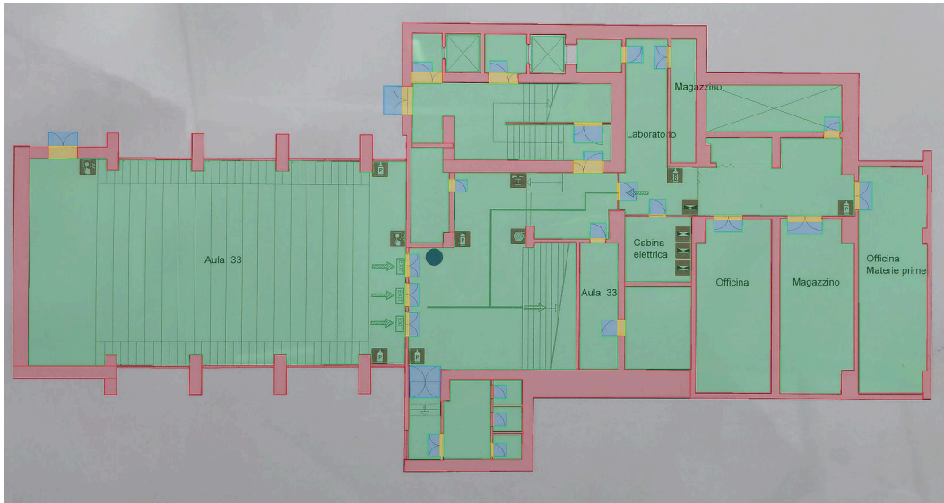
Figure 1.4 Output of the backend inference pipeline overlaid on the original floor plan image. Extracted architectural elements are converted into structured polygons, showing merged wall structures in red, flood-filled navigable rooms and corridors in green, and door openings in blue and yellow.
