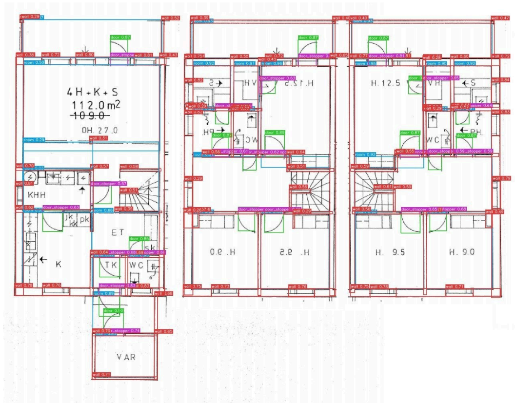
Figure 1.3 Raw output of the detection model of a floor plan, before geometric post-processing and human review in the frontend editor.
